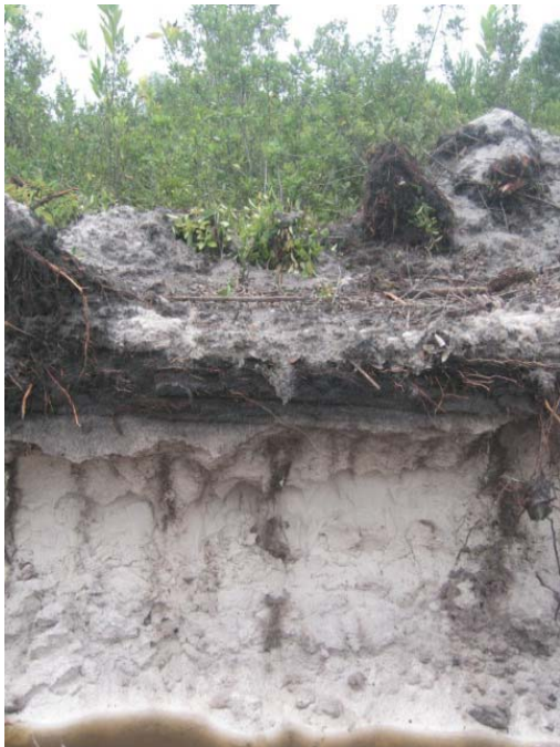
Figure 10: Shallow peat layer and sandy soil below, so called podzol. Secondary growths of bushes are seen in the rear.
