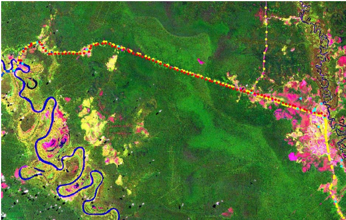
Figure 5: Landsat image RGB=543 acquired on 30.06.1991. On the left side is the Katingan river and on the right side the Rungan river. North is always up. The different green colours in the map show different PSF types. Yellow is the track on the Kalimantan highway (transect) and red are the 91 peat drillings 200m from the highway every 500m. Turquoises are the Peat Rivers.
